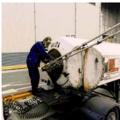
Driver wearing full face mask fitted with a filter. (Helmet removed for demonstrative purposes)
