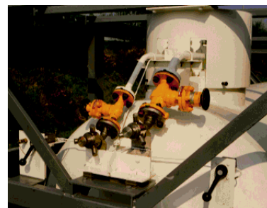
ISO tank container: detail of the connection point
