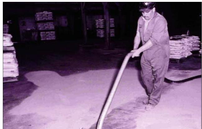
**Figure 7** Use of vacuum cleaning equipment
